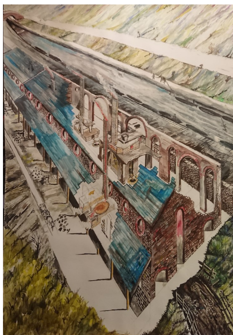
Image: Reconstruction of the Landore Copperworks, Swansea, and Morris Canal, c. 1790, copyright Stephen Hughes.
